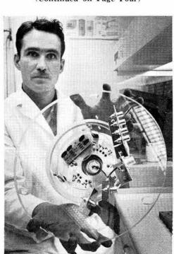
INSTRUMENTED TARGET for impact testing is displayed by Bob Hardy. Material to be tested (with flat surface facing projectile) is mounted on the other side of the quartz gage located in the center of the target mounting.
